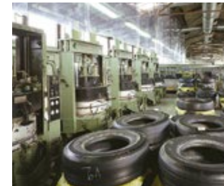
UBO: Hot-remould plant.
