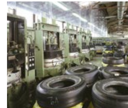
UBO: Hot-remould plant.
